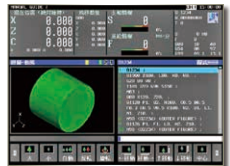
Cutting paths on single part in MGI
