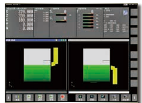
Cutting paths on 2 parts in MGI
