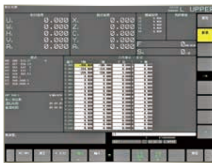
Tool offset setting & display
